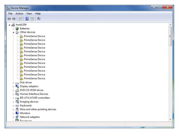
The exclamation point at "PrimeSense Device" informs that the required driver software has not been installed yet. This will be performed in the following software setup.
