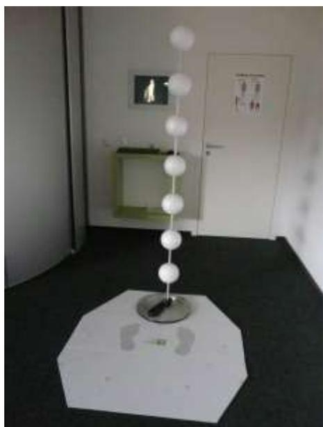
In the first step the calibration chain needs to be placed into the front position of the scan area. The button “Start Scan” starts the data acquisition.
